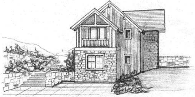
Retaining walls help blend building platform into natural topography
